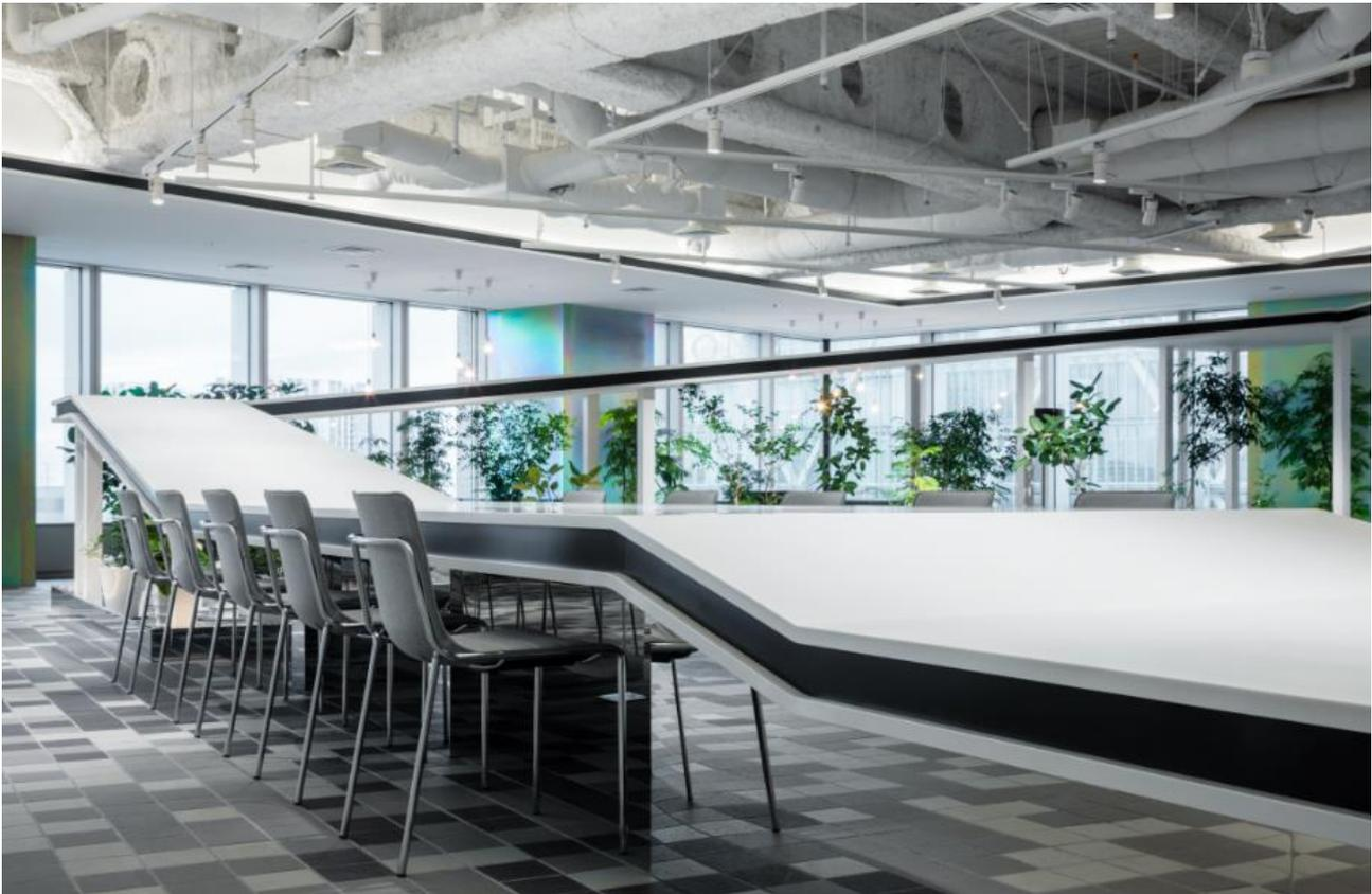
The “Storying” made from Corian® seems to be floating in space. This sense is created with legs made from mirrored stainless steel that reflect the floor tiles.
