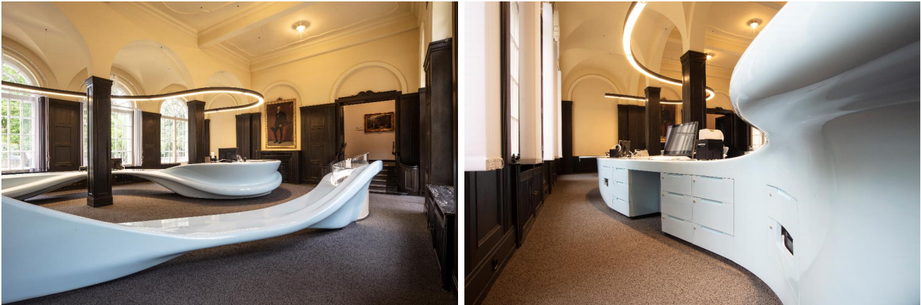
The counters of the Bad Kissingen Tourist Information centre were created on behalf of Bayerisches Staatsbad Bad Kissingen GmbH, and, thanks to the expertise of companies Grabner Design and Moser GmbH, are assembled from 4500 components made of Corian® Solid Surface. Concept / project / implementation: archicult - breunig architekten, Photo: Michael Stephan, all rights reserved.
